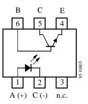
Figure 6. With base connection
