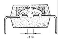
Figure 4. Cut through of a TEMIC optocoupler (thickness through insulation)
