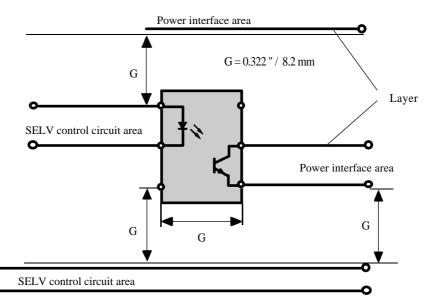
Figure 3. Top view of optocoupler mounting on a board (clearance on PC board: 0.322 "/ 8.2 mm, creepage path on PC board is 0.322 "/ 8.2 mm) Not only the solder eyes of the coupler itself on the board must have the 8-mm distance, but also all layers located between the SELV areas and the power interface areas.
