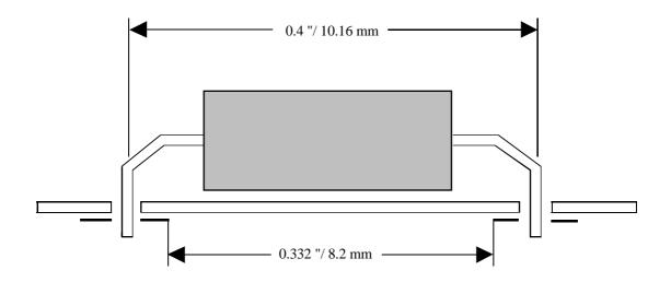
Figure 2. Optocoupler mounting on a board (side view)
