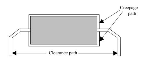
Figure 1. Isolation creepage/ clearance path
